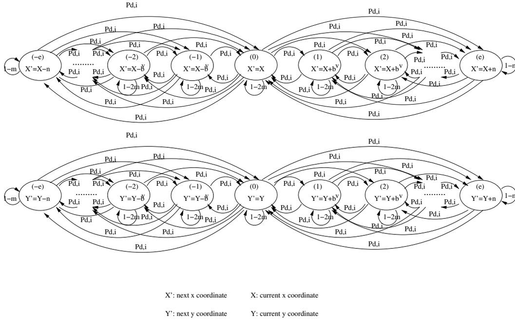
Fig. 6. State transition diagram for Model GIMM
