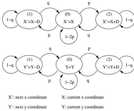
Fig. 3. State transition diagram for the SIMM model
